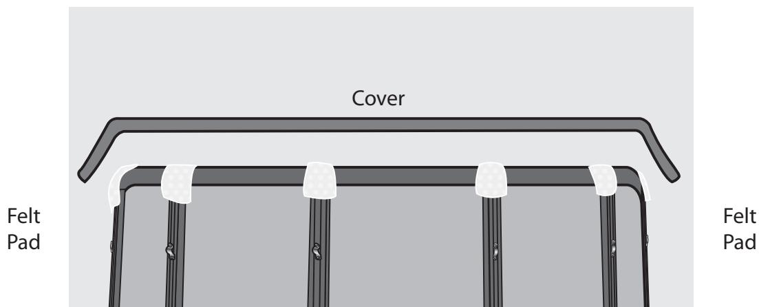
5 With the cover on and the pad in place attach a bungee cord around every upright. Continue to drill the straps at the set level pre-determined, judgement calls can be made at this point to ensure the cover is not too tight! There should be very little to no tension on the bungee cords at this point.
